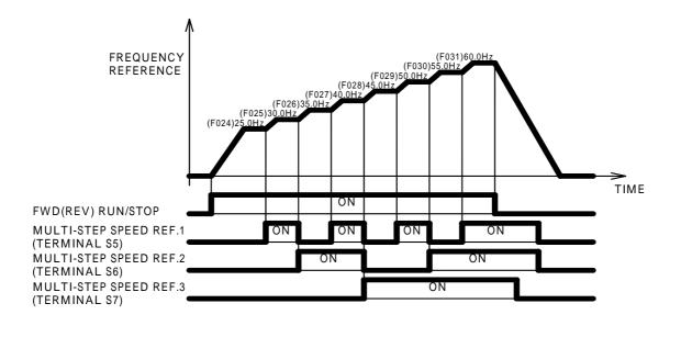
F050=1 (Input terminal S1) F051=2 (Input terminal S2) F052=3 (Input terminal S3) F053=5 (Input terminal S4) F054=6 (Input terminal S5) F055=7 (Input terminal S6) F056=8 (Input terminal S7)
