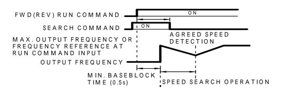
The deceleration time of speed search command can be set F101. If the setting is 0 sec., the inverter will still have 2.0 sec. as speed search time. When inverter output current is larger or equal to speed search current level (F102), speed search command starts.
