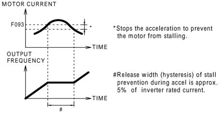
In the constant output area [output frequency max. voltage output frequency (F013)], following equation automatically decreases the stall prevention (current limit) level during acceleration.
