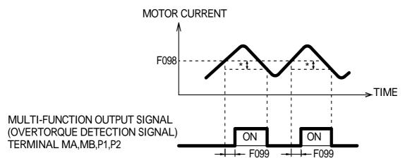
\*Overtorque detection release width (hysterisis) is set at approx. 5% of inverter rated current.
