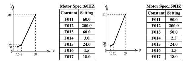
Increasing voltage of V/F pattern increase motor torque, but an excessive increase may cause :
