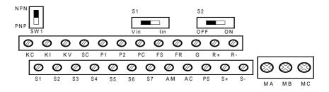
When connecting sequence inputs (S1~S7) with transistor, turn the rotary switch S1 depending on the polarity (OV common: NPN side, 24V common: PNP side). Factory setting: NPN side.
