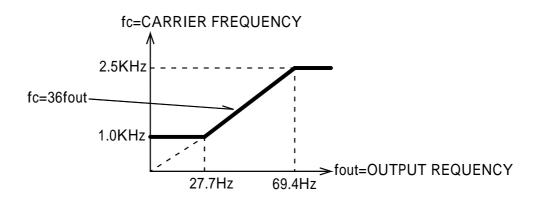
Factory setting varies according to inverter capacity.
