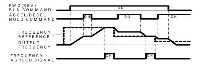
\* When the FWD (REV) run command is input along with the accel/decel hold command, the motor does not operate. However, when frequency reference lower limit (F034) is set greater than or equal to min. output frequency (F016), the motor operates at frequency reference lower limit.
