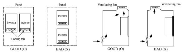
[When installing several inverters in a panel]
