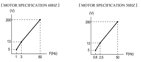
When operating with frequency larger than 60HZ/50HZ, change only max. output frequency (F011).
