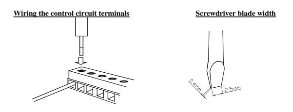
Insert the wire into the lower part of the terminal block and connect it tightly with a screwdriver.
