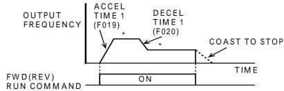
\*When frequency reference is changed during running. Upon removal of the FWD (REV)run command, the motor starts coasting.
