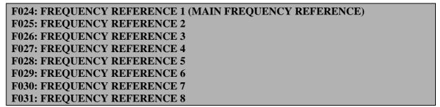
By combining frequency reference and input terminal function selections, up to 16 steps of speed can be set.
