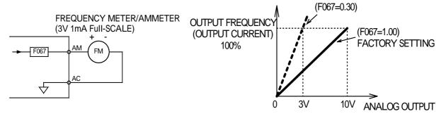
Example: Set the analog output voltage at 100% of output frequency (output current). Frequency meter displays 0 to 60Hz at 0 to 3V. 10 F067 setting (0.30)=3V.
