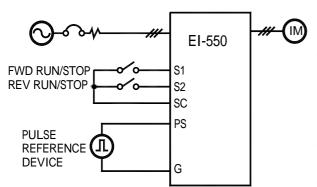
Run/Stop and FWD/REV can be selected by a switch of multi-function terminal input terminal S1, S2 for forward run/stop (F050=1), Reverse run/Stop (F051=2).
