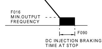
When coasting to a stop is specified in stopping method selection (F005=1), DC injection braking at stop does not operate.
